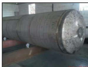
Sipchem Fluor -Vent Stack 40" 60M (SS)
