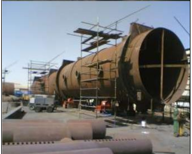
Fabrication of 120 ton Suffer Converter Vessel through INMA Steel Industry for ARAMCO – Khursaniyah Project
